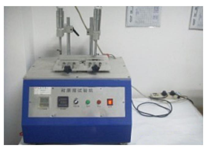
Rub-resistance test for colour fading
